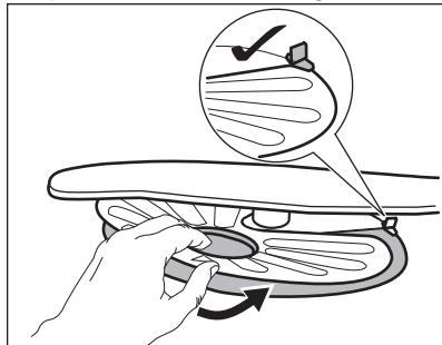
7. Reassemble the filters (B) and (C).
