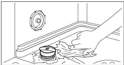
5. Turn the cap of the salt container clockwise to close the salt container.
